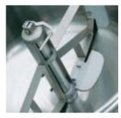
One mixing tool with lift off scrapers for all kind of mixing. Light but strong, unique shape.
